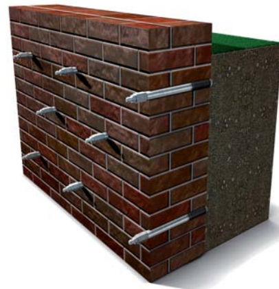
packer placement on brickwork
