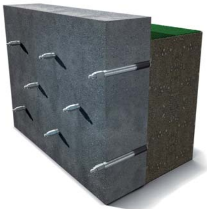
packer placement on concrete surfaces
